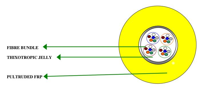
b. The typical construction of FTTH Cables (Polyethylene) is as follows:
