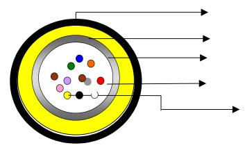
POLYETHYLENE SHEATH PULTRUDED FRP LOOSE TUBE THIXOTROPIC JELLY OPTICAL FIBRE
